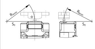
$R_{\mbox{\tiny Amin}}$  and  $R_{\mbox{\tiny Bmin}}$  depend on the actuator. Applies accordingly also to lateral retraction directions.
